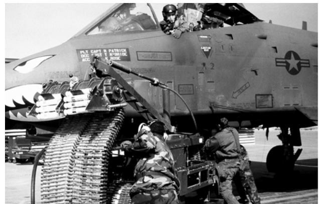
Figure 2.39. Loading Up an A-10.
